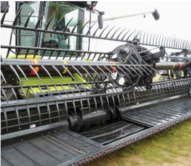
Draper fronts with some modifications are well suited to harvesting windrowed crops as well as for direct harvesting. PHOTO: P. CARMODY, DAFWA
