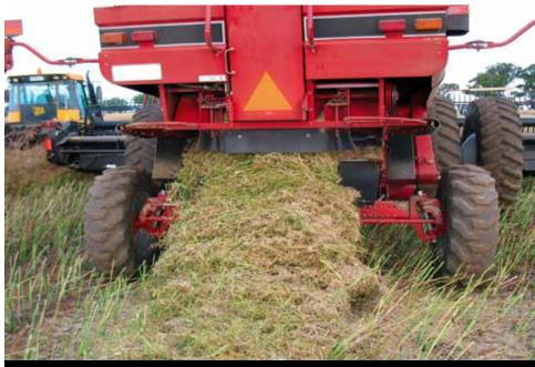
Canola can be quite green when harvested but is not hard to thrash. Rotor or drum speed should be about half to two-thirds of wheat speed, set at 450 to 650 revolutions per minute, and the concave should be set as wide as possible so stalks are not mashed up and overload the sieves.
